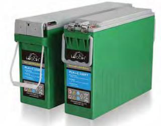
LEOCH Pure Lead Carbon Front Terminal batteries, PLH+C series, are AGM Valve-Regulated Lead-Acid front terminal batteries that have been optimized for hybrid telecom applications. Engineered for long life shallow cycling applications such as Hybrid and Renewable Energy powered Base Transceiver Stations. PLH+C batteries offer long life design and high cyclic performance.
