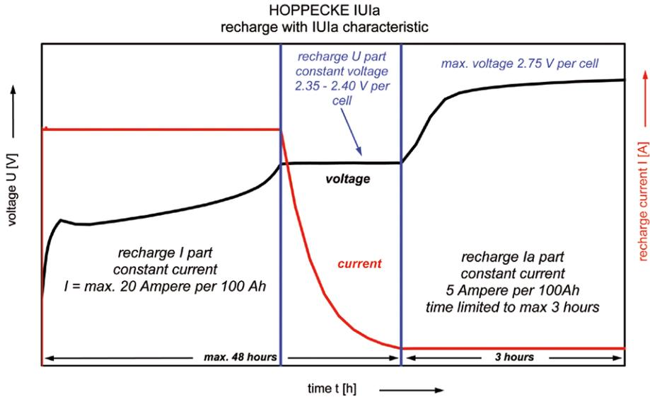
Fig. 9-2: IU<sub>a</sub> characteristic
