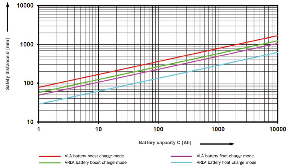
Fig. 5-1: Safety distance based on battery capacity
