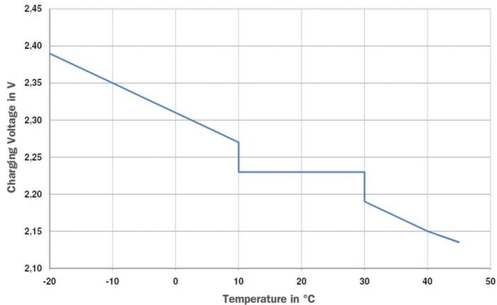
Fig. 6-1: Temperature related float charge voltage adjustment
