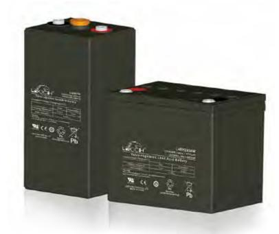
LEOCH LHR series, are AGM Valve-Regulated Lead-Acid front terminal batteries that have been optimized for UPS applications. Engineered to offer high-power discharge rates at 15mins and high consistency for multiple string applications, LHR batteries offer an up to 16-year (2V) and 12-year (12V) life design and a wide 12V and 2V capacity range to cover any requirement.
